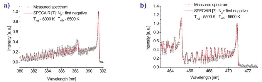
Comparisons of the measured and simulated emission spectra of N<sub>2</sub>+ first negative system (for two different bands) in nitrogen plasma ( $P_A = 2$  kW, nitrogen flow rate - 50 l/min, 25 mm below the electrode end)
