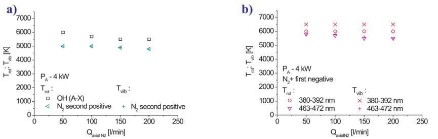
Measured rotational and vibrational temperatures of OH radicals, N<sub>2</sub> molecules (a) and N<sub>2</sub>+ ions (b) as a function of axial nitrogen flow rate  $Q_{axialN_2}$  ( $P_A = 4$  kW, 25 mm below the electrode end)
