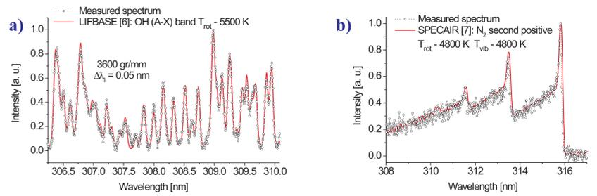
Comparison of the measured and simulated emission spectra of OH(A-X) rotational band and N<sub>2</sub> second positive system in nitrogen plasma ( $P_A = 2$  kW, nitrogen flow rate - 50 l/min, 25 mm below the electrode end)
