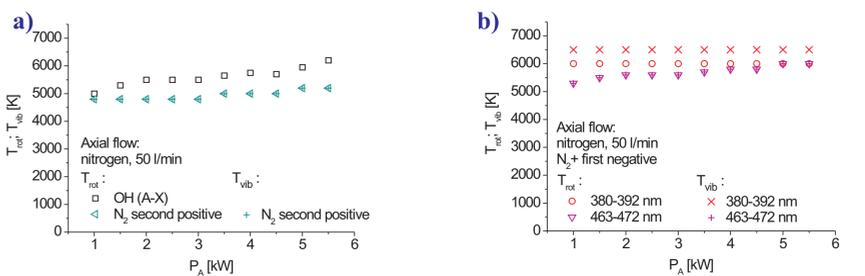
Measured rotational and vibrational temperatures of OH radicals, N<sub>2</sub> molecules (a) and N<sub>2</sub>+ ions (b) as a function of microwave absorbed power  $P_A$  (nitrogen flow rate - 50 l/min, 25 mm below the electrode end)
