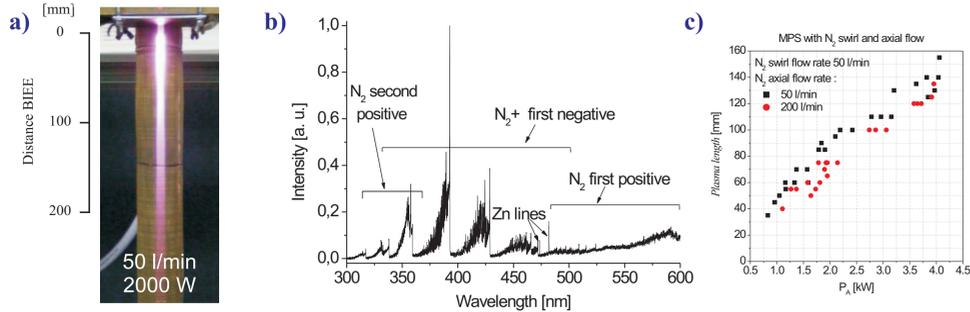
a) Nitrogen microwave plasma, b) Measured emission spectrum of nitrogen plasma ( $P_A = 2$  kW, nitrogen flow rate - 50 l/min, 25 mm below the electrode end) c) the length of nitrogen plasma (measured from electrode) as a function of microwave absorbed power  $P_A$  ( $P_A = P_i$  (incident) -  $P_r$  (reflected)) for different axial flow rates
