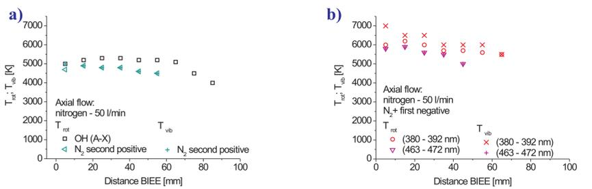
Measured rotational and vibrational temperatures of OH radicals, N<sub>2</sub> molecules (a) and N<sub>2</sub>+ ions (b) as a function of distance below inner electrode end (Distance BIEE) ( $P_A = 2$  kW, nitrogen flow rate - 50 l/min)
